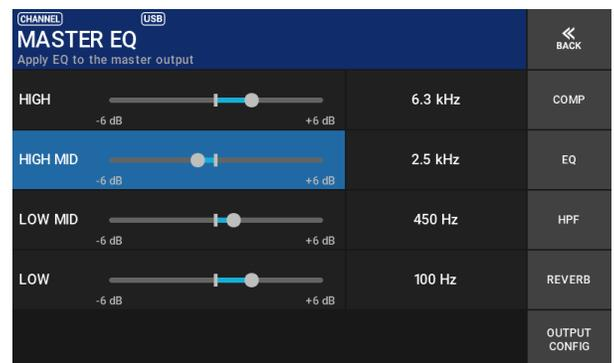
The HIGH and LOW bands are a shelving EQ with a Q of 0.707. The MID bands are a peak/dip EQ with a Q of 1.5.
