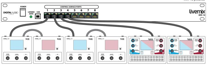
Each Control Surface Port on the MIX-16/MIX-32 supports either two CS-SOLOs or one CS-DUO. Connect the CS PORT IN on a CS-SOLO to a Control Surface Port on the MIX-16/MIX-32. If using a second CS-SOLO, connect the CS Port Thru on the first CS-SOLO to the CS PORT IN on the second CS-SOLO. See Connecting Two CS-SOLOs
