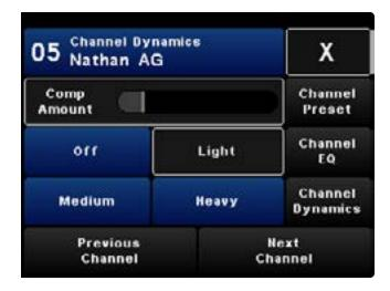
PRESS any of the 4 buttons at the bottom of the screen to select how much compression is needed.
