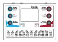
The CS-DUO supports two mixes. To set up the CS-DUO, connect a CAT5e or CAT6 cable (shielded recommended) from the CS-DUO to an available Control Surface Port on the MIX-16/MIX-32. Please note, only one CS-DUO can connect to a CS Port on the MIX-16/MIX-32. You cannot connect a CS-DUO to the CS Port Thru on a CS-SOLO.
