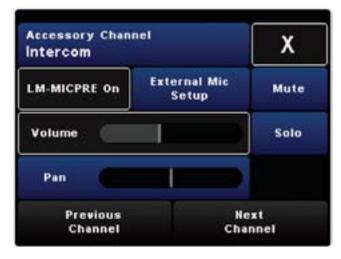
**NOTE**: If some users are using the built-in intercom and some are using external microphones, you may need to adjust the gain knob on the LM-MICPRE to match respective intercom volume levels.
