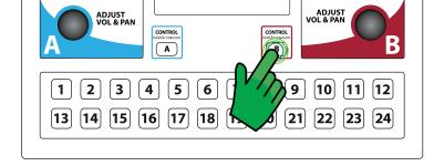
appropriate color. All channel select buttons, knobs and touchscreen controls are assigned to the selected mix.
